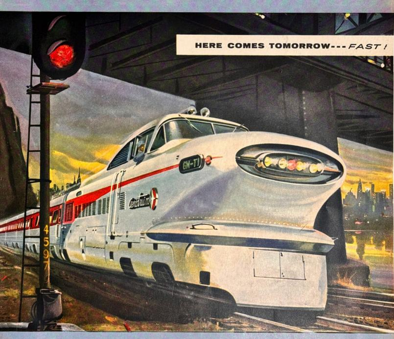
THE TWO new lightweight General Motors Aerotrains are about to start their tour of American railroads. This great Electro-Motive development might well revolutionize travel by rail. With steel underframe and aluminum body, the 100-mile-an-hour Aerotrain is 50% lighter than conventional trains. It costs much less to build and much less to operate. It is Electro-Motive's current contribution to the thinking designed to win passenger traffic for railroads—and help to make it profitable.
