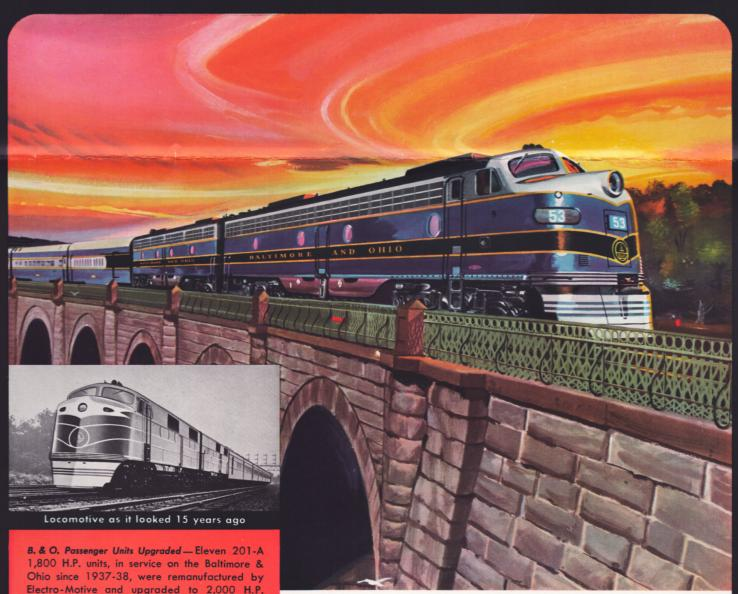
1,800 H.P. units, in service on the Baltimore & Ohio since 1937-38, were remanufactured by Electro-Motive and upgraded to 2,000 H.P. These modernized 17-year-old General Motors locomotives have gone back into the passenger pool handling regular runs with the same effi-
