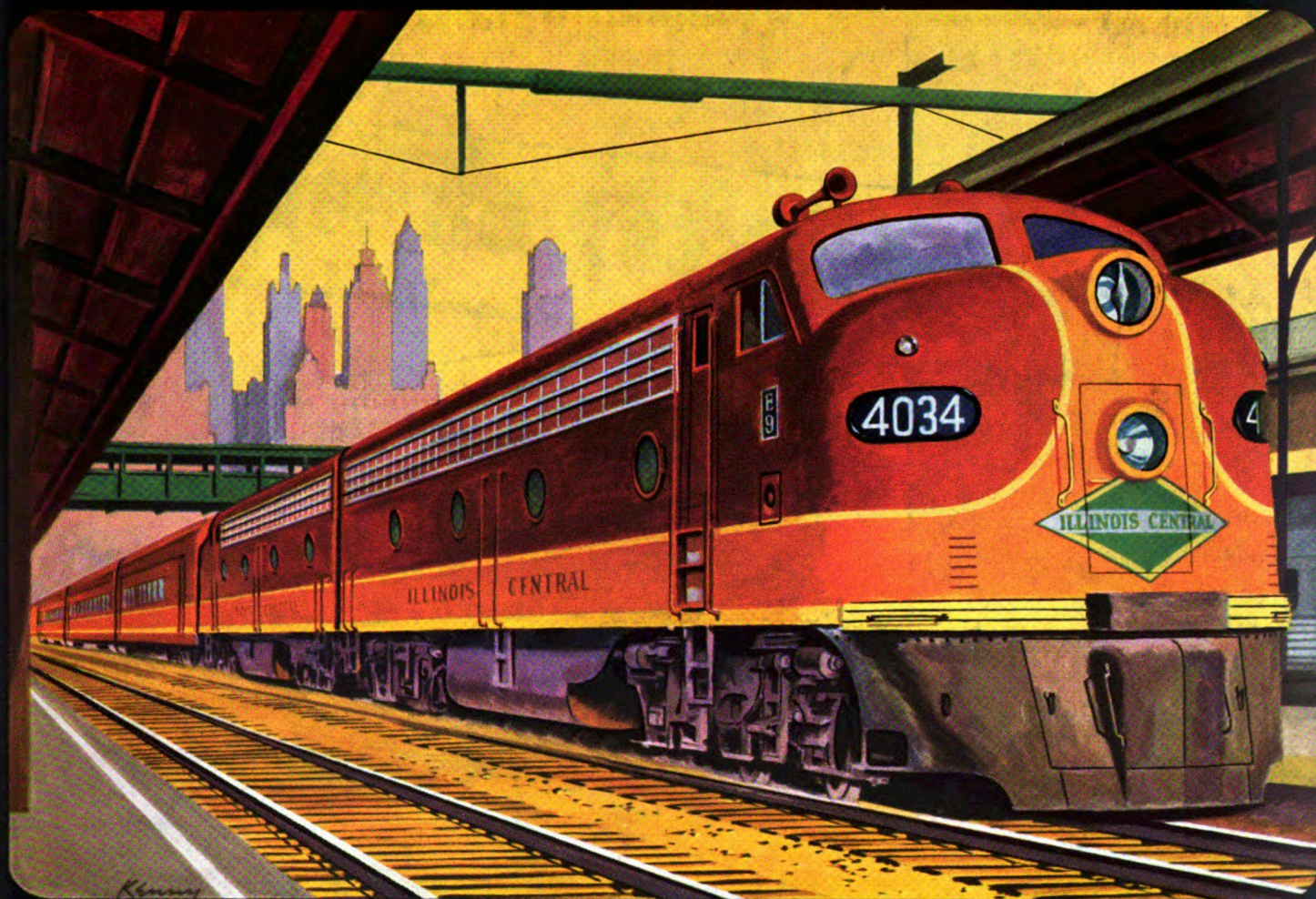
New 2400-Horsepower E9 Passenger Units Delivered to Illinois Central
