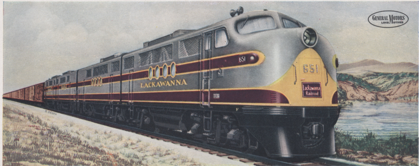
5400 H.P. DIESEL FREIGHT LOCOMOTIVE . . DESIGNED AND BUILT BY ELECTRO-MOTIVE DIVISION . . GENERAL MOTORS CORPORATION . . LA GRANGE, ILLINOIS, U. S. A.
