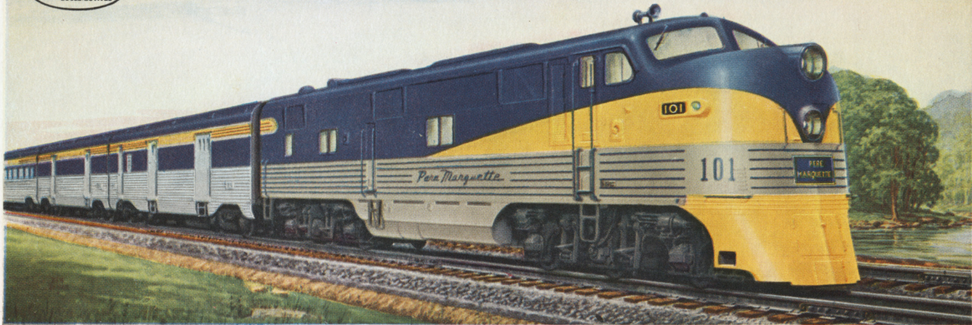
2000 H.P. DIESEL PASSENGER LOCOMOTIVE . . DESIGNED AND BUILT BY ELECTRO-MOTIVE DIVISION . . GENERAL MOTORS . . LA GRANGE, ILLINOIS, U. S. A.
