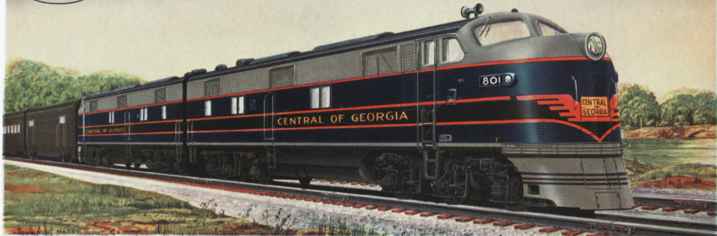
4000 H.P. DIESEL PASSENGER LOCOMOTIVE . . DESIGNED AND BUILT BY ELECTRO-MOTIVE DIVISION . . GENERAL MOTORS . . LA GRANGE, ILLINOIS, U. S. A.
