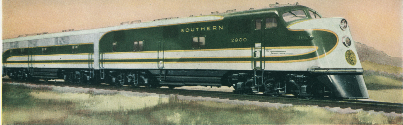
4000 H.P. DIESEL PASSENGER LOCOMOTIVE . . DESIGNED AND BUILT BY ELECTRO-MOTIVE DIVISION . . GENERAL MOTORS . LA GRANGE, ILLINOIS U. S. A
