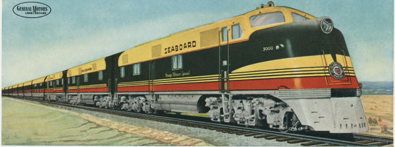
6000 H.P. DIESEL PASSENGER LOCOMOTIVE . . DESIGNED AND BUILT BY ELECTRO-MOTIVE DIVISION . . GENERAL MOTORS . LA GRANGE, ILLINOIS, U. S. A.
