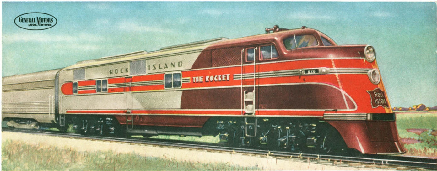
2000 H.P. DIESEL PASSENGER LOCOMOTIVE . . DESIGNED AND BUILT BY ELECTRO-MOTIVE DIVISION . . GENERAL MOTORS . . LA GRANGE, ILLINOIS, U. S. A.
