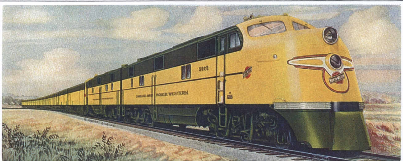
4000 H.P. DIESEL PASSENGER LOCOMOTIVE . . DESIGNED AND BUILT BY ELECTRO-MOTIVE DIVISION . . GENERAL MOTORS CORPORATION . . LA GRANGE, ILLINOIS, U. S. A.
