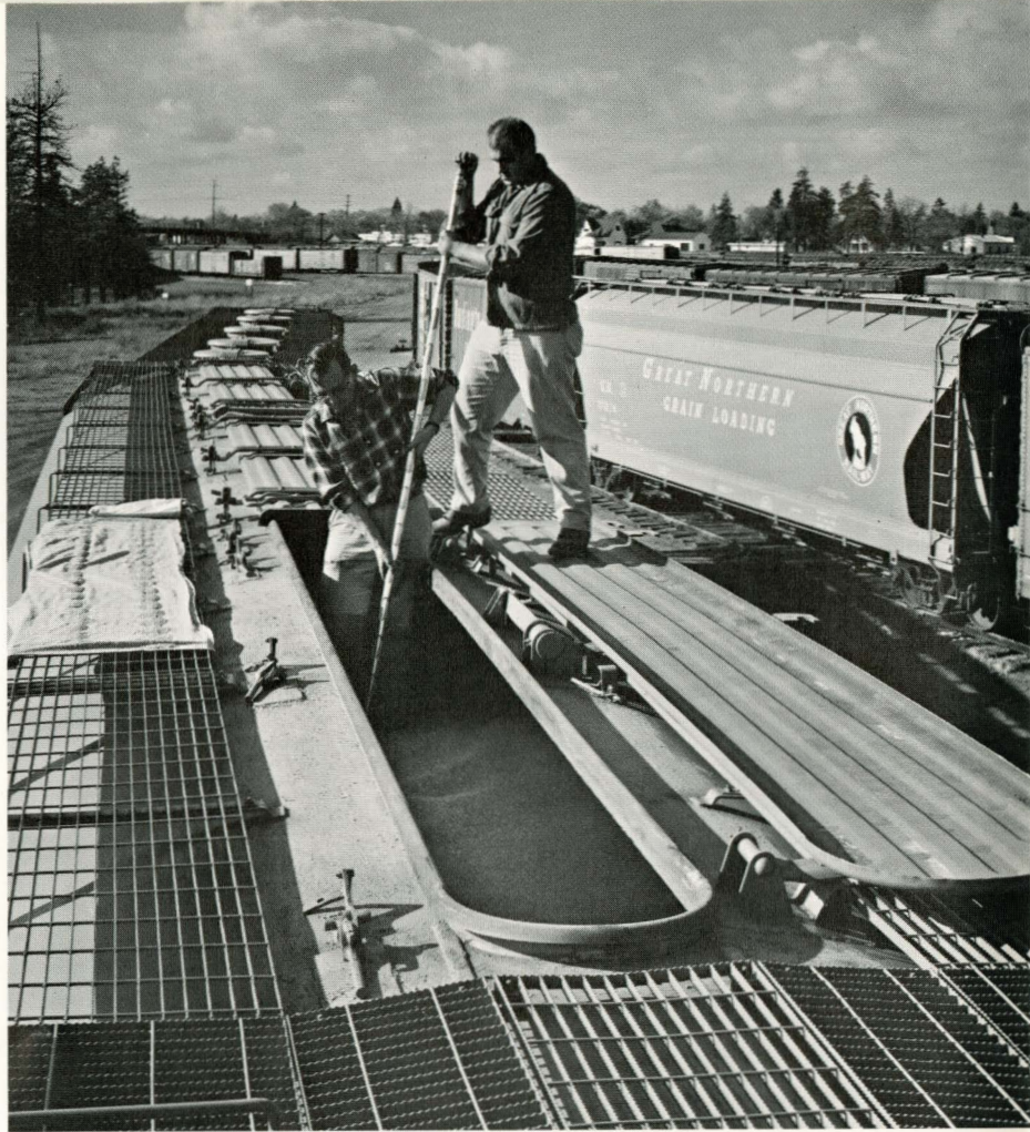
Washington State grain inspectors at Spokane take a wheat sample from a new GN "jumbo" covered hopper. These efficient cars carry half again as much grain as the average box car and are much more quickly loaded and unloaded. We added 300 to our fleet in 1965 and will acquire another 300 during 1966.
