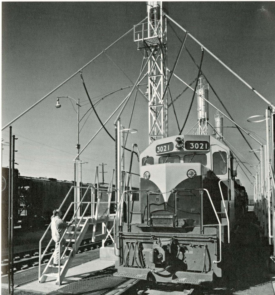
Pausing briefly between runs at Hillyard Yard in Spokane, this big 2500 HP freight diesel gets fuel, water, sand and a quick scrub-down. Locomotives of this type averaged better than 13,000 miles of service monthly in 1965.
