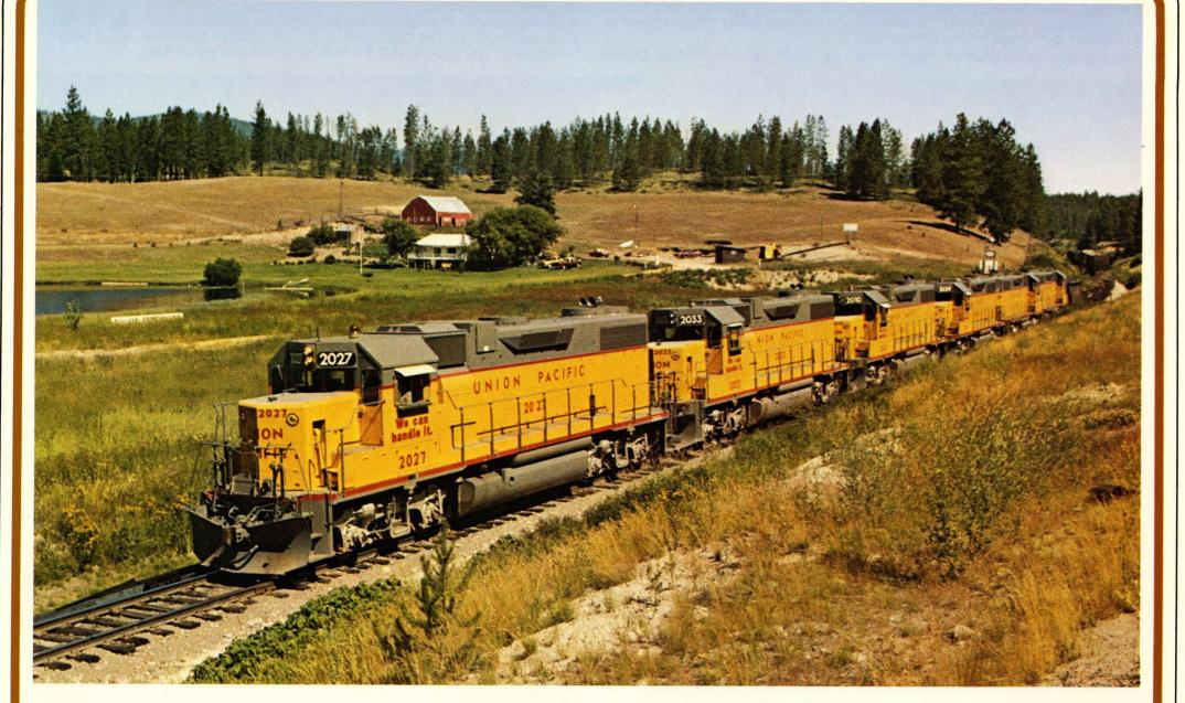
**GP-38-2** The 2,000 horsepower GP-38-2 weighing 269,460 pounds is capable of a maximum speed of 70 miles per hour. The length of this unit is 59 feet, 2 inches, height is 16 feet.
