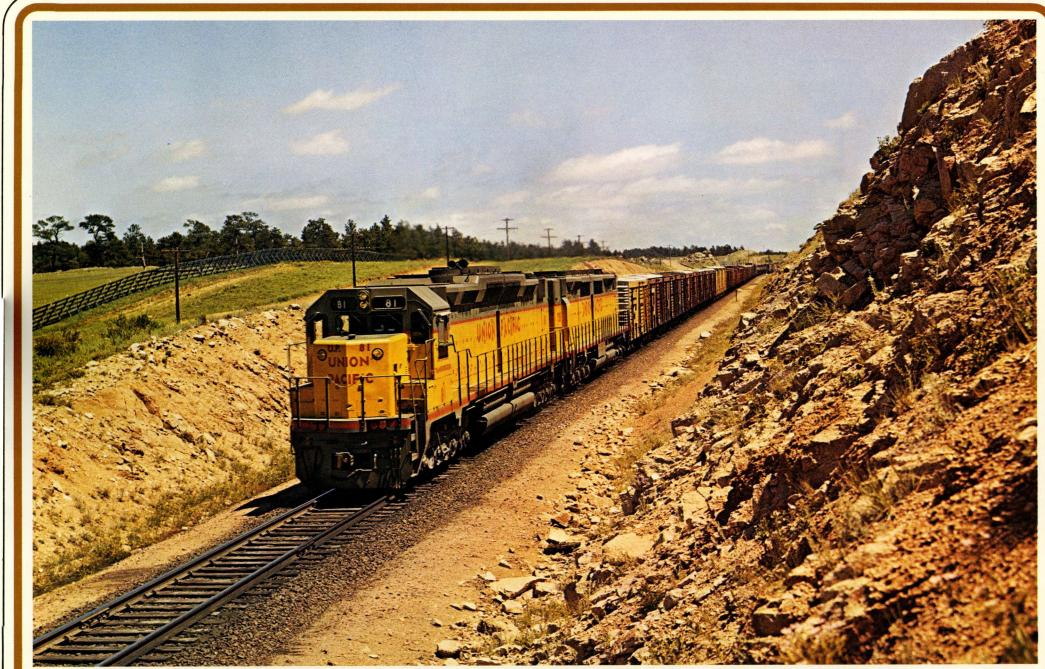
**DD-35A**The DD-35A weighs 521,980 pounds and is capable of a maximum speed of 90 miles per hour. Measuring 17 feet, 2½ inches in height, this 5000 horsepower locomotive is 88 feet, 2 inches long.
