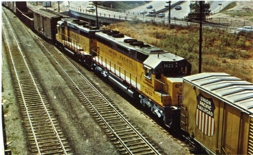
Mid-train robot locomotive . . . operated through control console in master unit. (shown above)
