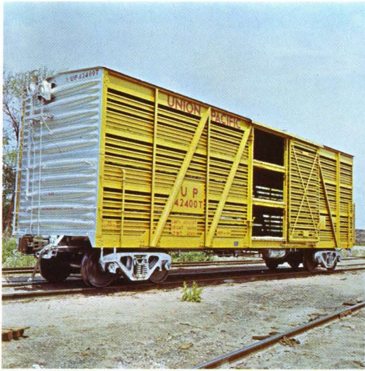
New triple-deck livestock car will transport 40 tons of hogs or sheep.
