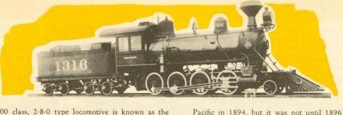
The 400 class, 2-8-0 type locomotive is known as the "Consolidation" type. Type 2-8-0 stands for the wheel arrangement under the locomotive, that is, there are two forward truck wheels, eight driving wheels, and no trailing truck wheels on this locomotive. This designation is used universally in the United States to distinguish different railroad motive power.
