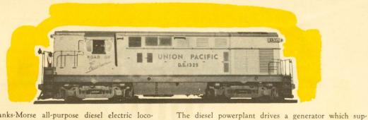
The Fairbanks-Morse all-purpose diesel electric loco-motive is an 0-4-4-0 type of 1500 HP, a number of which have recently been placed in service of Union Pacific. This type is also known as a "road-switcher" since it can be used in the dual role of switching locomotive
