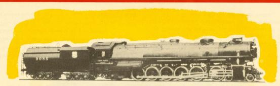
The 9000 class, 4·12·2 type locomotive is known as the "Union Pacific" because it was designed by the Engineering Department of the Union Pacific Railroad at Omaha. It was first placed in service in 1926 and has remained a mainstay of steam motive power on the railroad for over two decades.
