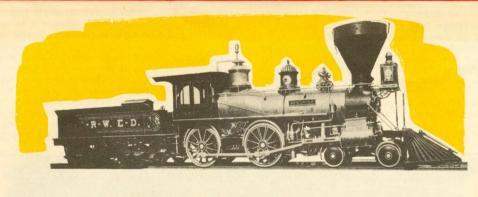
Locomotive No. 22 was built in 1875 by Baldwin Locomotive Works and was known as an "eight-wheeler". The drive wheels are 57 inches in diameter and it operates with a boiler pressure of 130 pounds. This speedy woodburner of yesteryear stands 14 feet
