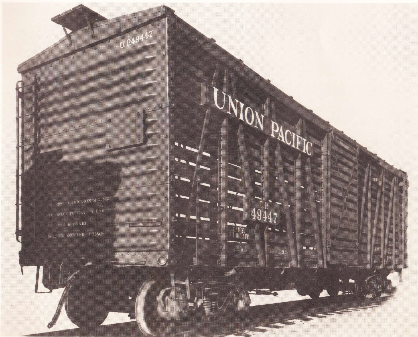
Stock Car, used to ship cattle, horses and mules. Similar cars, double-decked, carry hogs and sheep. Every 36 hours stock must be unloaded for water, feed and rest. Stock cars are placed at head end of train.
