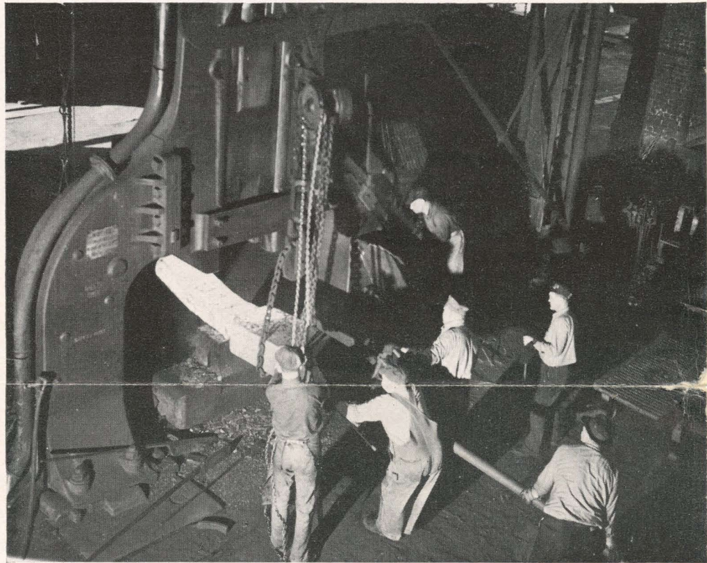
These S. P. workmen are forging a heavy steel locomotive part with a giant 10,000-lb. steam hammer. Since Aug. 1, 1939, S.P. has ordered 252 locomotives!
