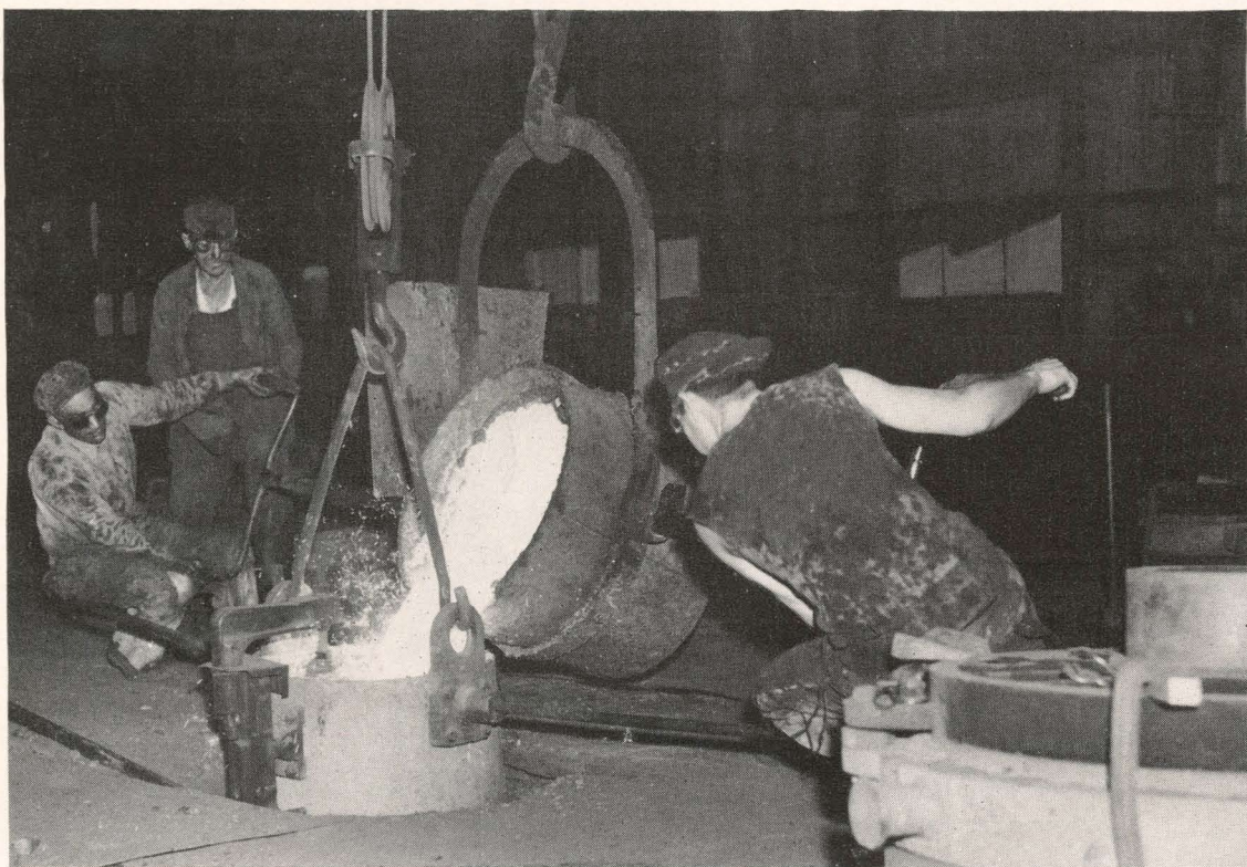
Moulders below are pouring a bucket of hot stuff in the wheel foundry of the Sacramento Shops. Southern Pacific makes a great deal of its own equipment, does its own repair work.
