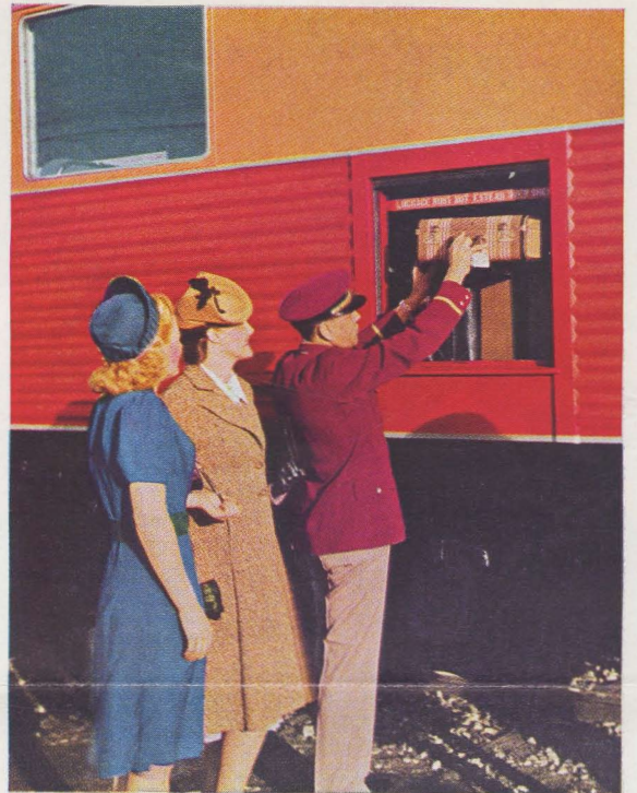
Baggage Elevators are a Southern Pacific innovation on the San Joaquin Daylights . Baggage is stored here so passengers do not have to wait in the aisles while it is being unloaded.
