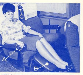
HERE'S HOW TO OPERATE YOUR CHAIR .... (A) This trigger on arm controls back of seat. Pull up on trigger and push seat back to position desired. When seat is reclined pull up on trigger to bring back of seat forward.
