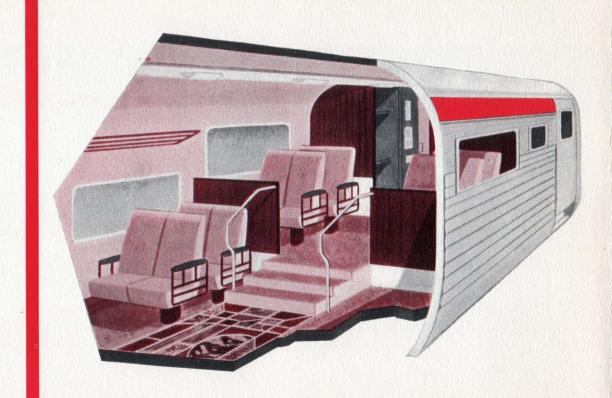
ARLY IN 1956 a train of "rail-hugging" two-level passenger cars shown on the cover will go into service on the Pennsylvania Railroad. Revolutionary new tubular design makes its center of gravity the lowest ever engineered for railroad cars, permitting faster schedules, increased passenger comfort, and sharply reduced construction, operating and maintenance costs.
