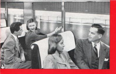
EXTRA-SPACIOUS WINDOWS—panoramic for wide-angle views. Six feet wide... divided in the center with a metal strip to provide an individual shade for each double seat. Double-paned to shut out noise, heat, cold and dust.
