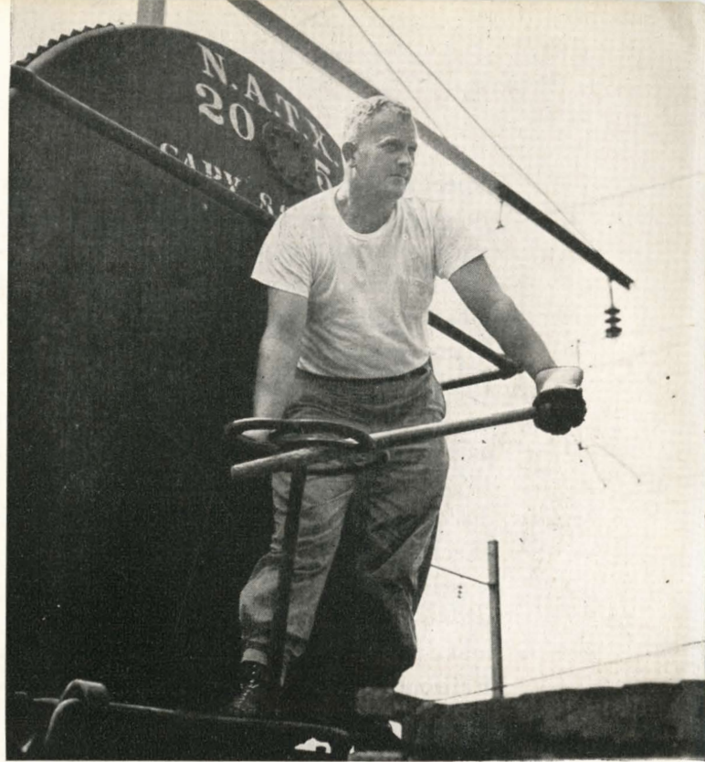
"Always couple at less than four miles an hour" is the slogan of the brakemen in Pennsylvania's careful handling campaign to reduce claims for damage to freight.
