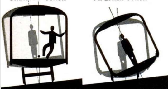
Ordinary coaches sway out on fast turns. The Xplorer's bank right into them. You can stand or walk with less lurching.
