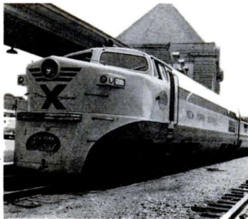
Xplorer's engine is a diesel-hydraulic unit. One to run on the New Haven will have electric motors besides, for tunnel use.
