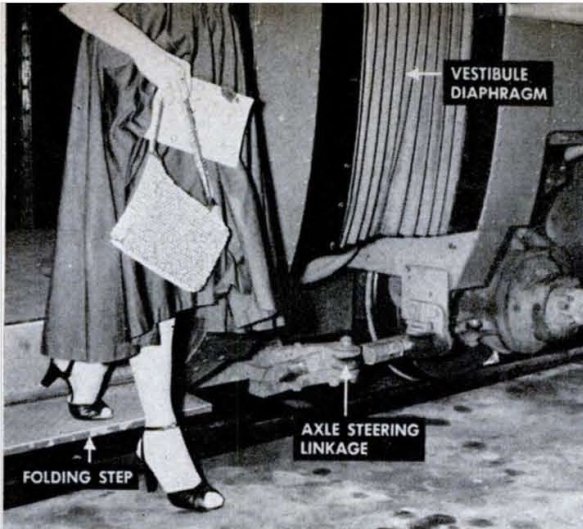
Sleek and low, coaches are fitted with folding steps. It's only two steps down to a low-level station platform like this.
