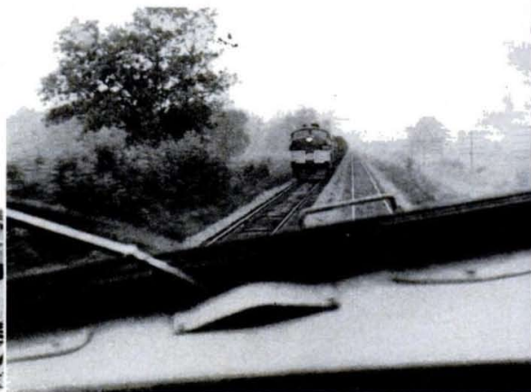
Fireman's-eye view shows the auto-like cowl of the new locomotive. Its cab is almost directly over the front wheels.
