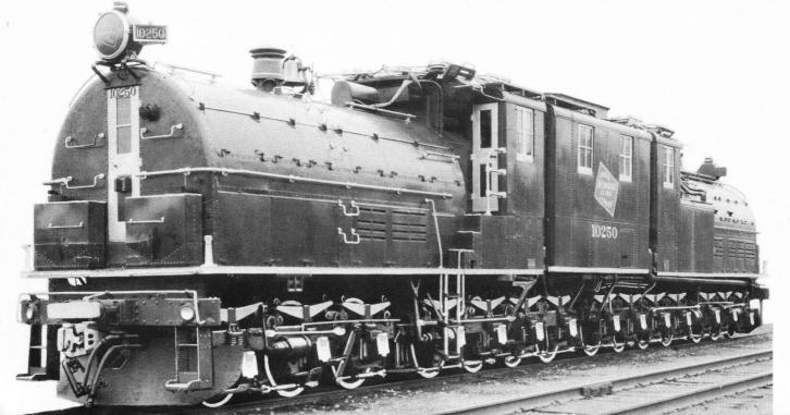
ELECTRIC LOCOMOTIVE No. 10250-BUILT IN 1919 by the General Electric Company and the American Locomotive Company. This is a bi-polar gearless motor and is the type used to haul passenger trains of The Milwaukee Road across the Cascade Mountains. This locomotive was renumbered E 1 in 1939.
