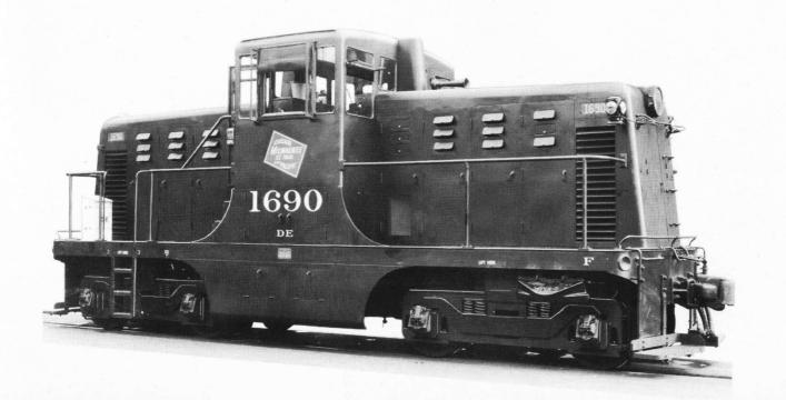
No. 1690—Built in 1940 by the General Electric Company. This is a 380 horse power, 44-ton switcher for light industrial switching. This locomotive has been re-numbered 1699.
