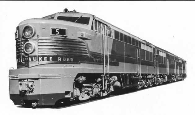
**DIESEL-ELECTRIC** Locomotive No. 5-BUILT IN 1946 by Fairbanks, Morse & Co. and the General Electric Company. The units of these locomotives can be coupled to make 4000 h.p. (2-unit) or 6000 h.p. (3-unit) locomotives. Each unit is equipped with a 2000 h.p. Diesel engine-generator which supplies electricity to four geared traction motors. The coupled length of each unit is 64 ft. 10 in.; total weight, 328,800 lbs.
