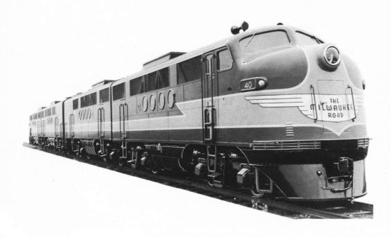
**No. 40**—Class DE-54—BUILT IN 1941 by the Electro-Motive Corporation. This four unit locomotive is rated at 5400 horsepower. Each of four Diesel engines drives an electric generator which produces 1350 horsepower at full load speed, 800 r.p.m. Traction motors are geared to 40-inch driving wheels.
