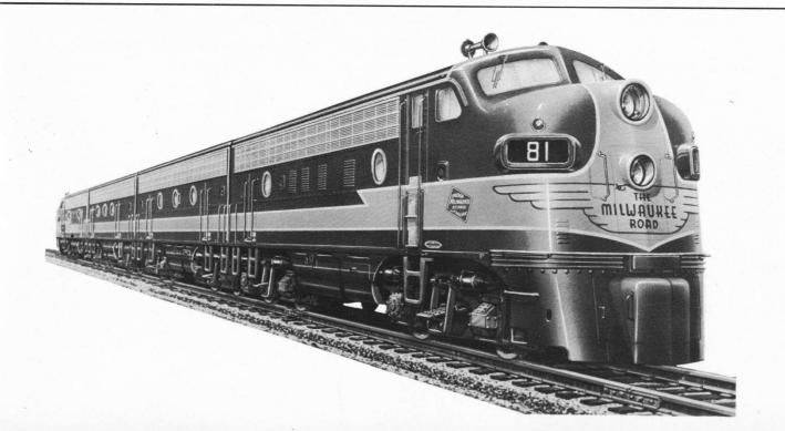
**DIESEL-ELECTRIC** Locomotive **No. 81**—Built in 1949 by Electro-Motive Division, General Motors Corporation. This is a 4-unit freight locomotive. Each unit is rated at 1500 horse power. It is equipped with dynamic brakes to control train speed on descending grades.
