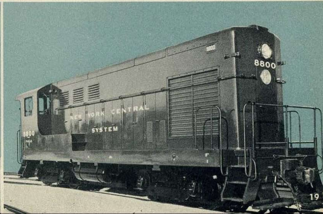
A 1,000-hp diesel electric switching locomotive.
