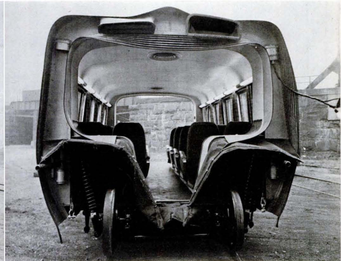
Rear view of car shows pins to support car behind it, coil-type springs, and outer strip that
