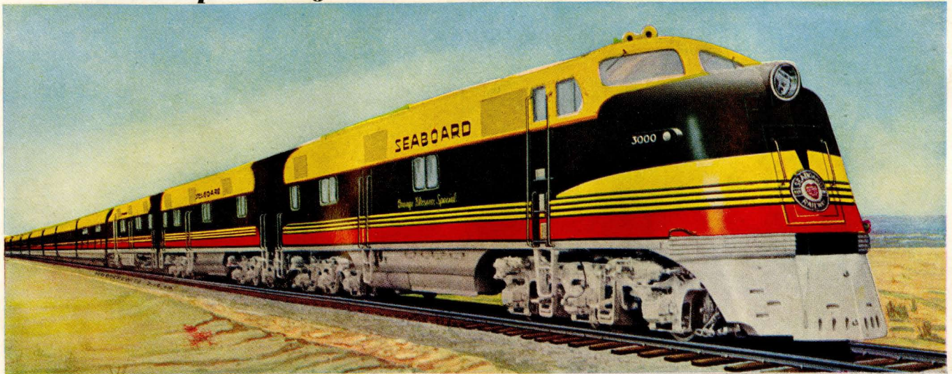
SEABOARD RAILWAY—6000 H.P. DIESEL PASSENGER LOCOMOTIVE
