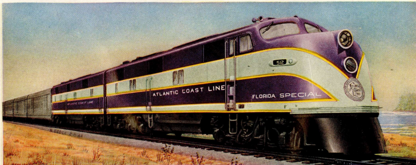
ATLANTIC COAST LINE—4000 H.P. DIESEL PASSENGER LOCOMOTIVE
