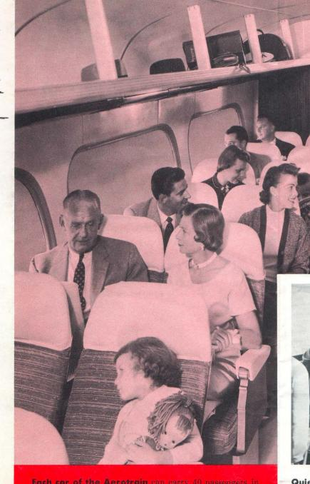
Each car of the Aerotrain can carry 40 passengers in double reclining seats, each with its own reading light. The GMC coach body has been widened 18 inches to give more comfortable seating space and a wider aisle. Each car is equipped with a lavatory and pantry space for assign light most.
