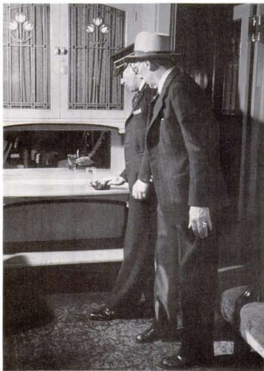
In an old-style car, a glass of water comes dangerously near to slopping over brim as the train goes around a curve. Notice the tilt of the water surface in the glass.
