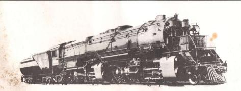
ing 2-8-8-2 was the all-time giant of Great Northern's steam fleet—and largest locomotive in the world when Baldwin built the first of its class. Most of the big R's, however, came from the railway's own shops at Hillyard, Washington, and were the first steam locomotives built in the Pacific Northwest. Heaviest and most powerful of two sub-classes was the R-2, pictured here. Overall
