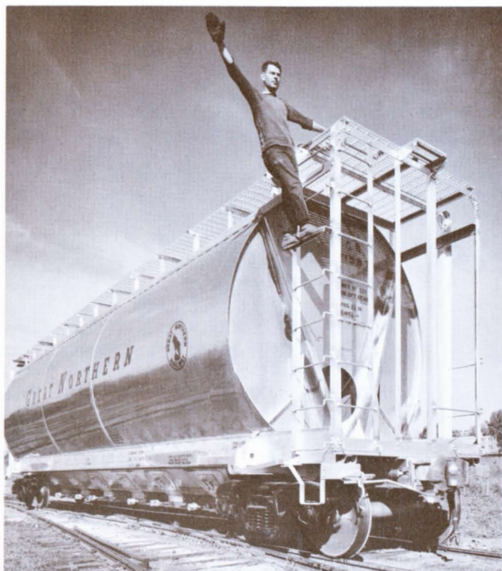
Designed for bulk commodities such as feed, grain and malting barley, these new "jumbo" aluminum hopper cars weigh far less than a conventional covered hopper but carry a greater payload.
