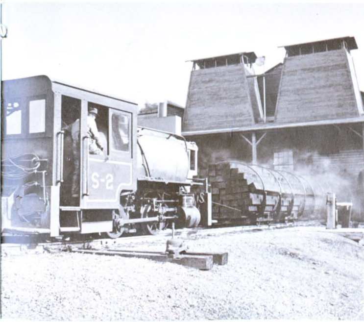
Somers Lumber Division of the Glacier Park Company, a GN subsidiary, operates a tree farm and this tie-treating plant at Somers, Montana, providing a large share of the treated crossties used by the railway.
