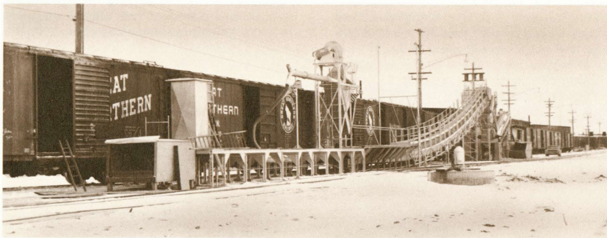
Cleaning of freight cars became speedier and more efficient with the completion in 1961 of Great Northern's new mechanized car-cleaning facility at Grand Forks, North Dakota.
