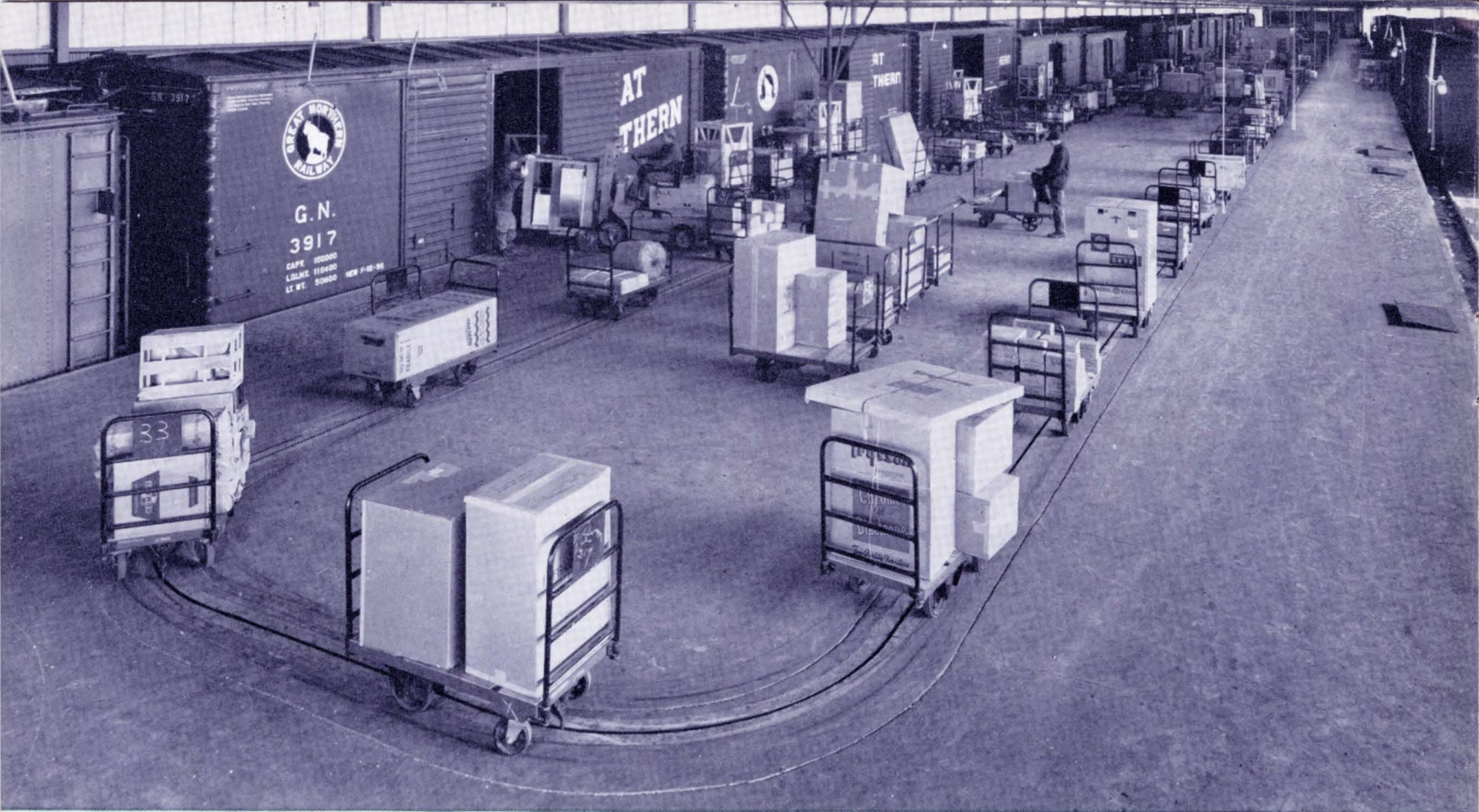
CONTINUOUS CONVEYOR CHAIN SPEEDS LOADING OF MERCHANDISE.
