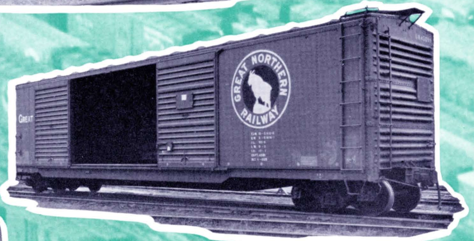
FIFTEEN FOOT WIDE DOORS PERMIT MECHANICAL LOADING OF LUMBER AND OTHER COMMODITIES.
