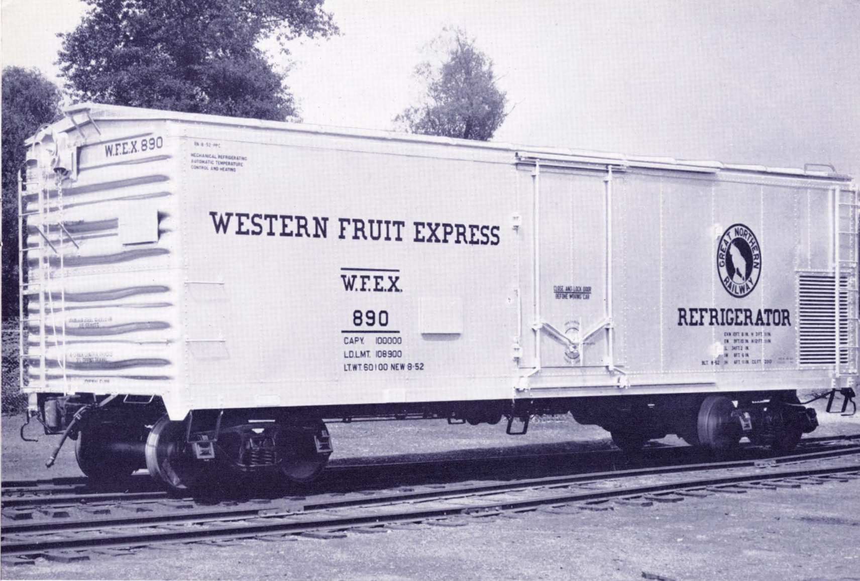
ALL-PURPOSE, HEAVILY INSULATED, MECHANICAL REFRIGERATOR CAR, CAPABLE OF MAINTAINING ANY FIXED INSIDE TEMPERATURE OF ZERO DEGREES OR OVER, BY FURNISHING HEAT OR COLD AS NEEDED. WESTERN FRUIT EXPRESS CO. IS A WHOLLY-OWNED SUBSIDIARY OF GREAT NORTHERN RAILWAY CO.
