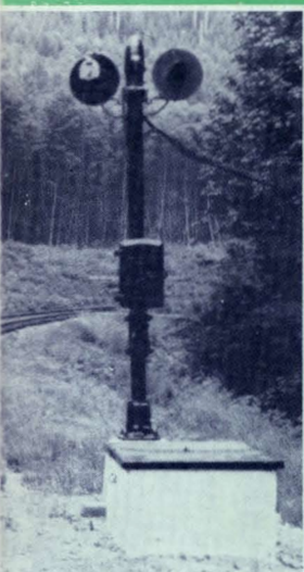
Dragging equipment detector and indicator located ahead of train
