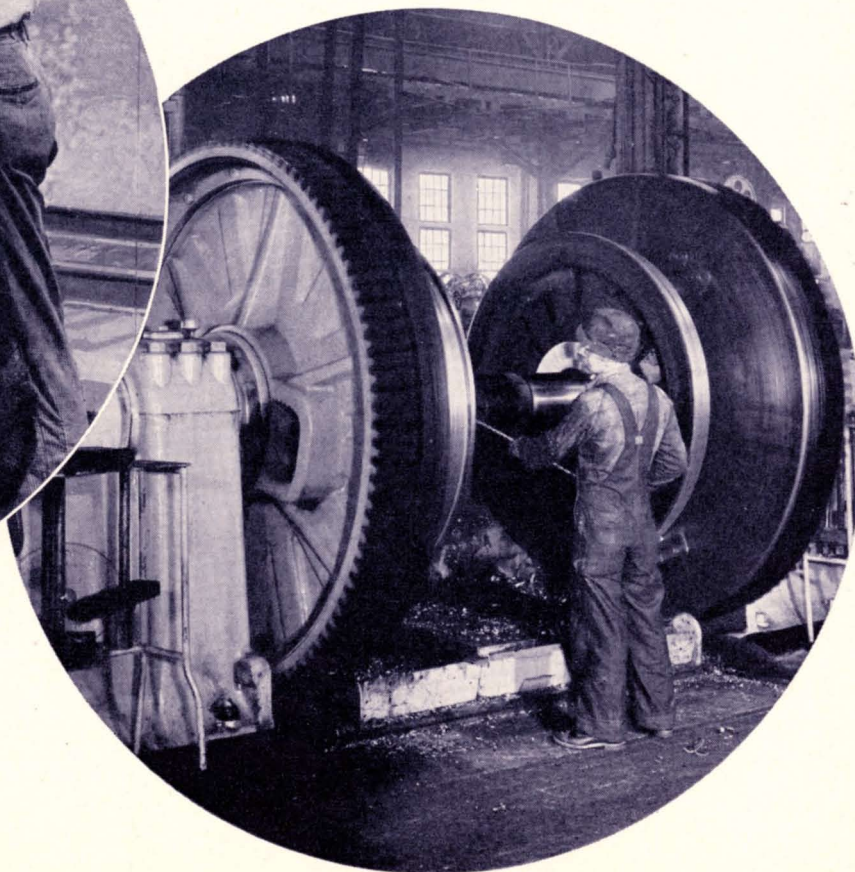
THIS 90-INCH WHEEL LATHE SPEEDS LOCOMOTIVE MAINTENANCE.
