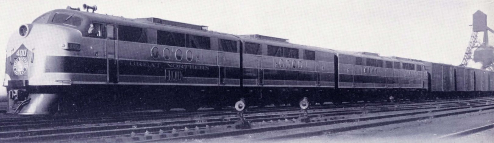
5400 HORSEPOWER DIESEL ENGINES HAUL FREIGHT TRAINS OVER ROCKY MOUNTAINS.
