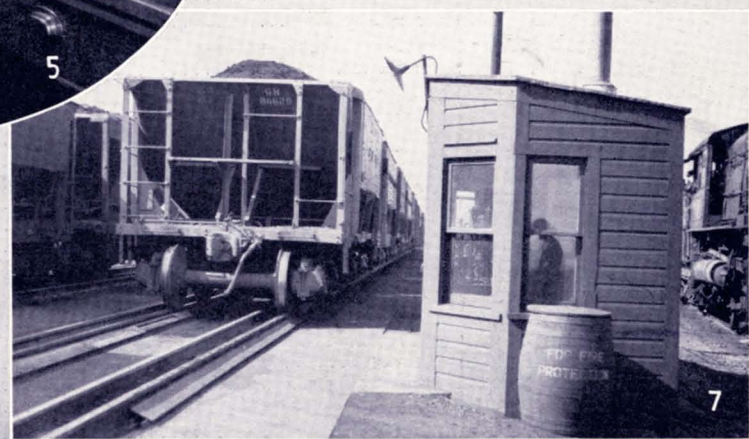
At dock yards—weighing and assorting cars according to grades of ore—requires 78 miles of track.
