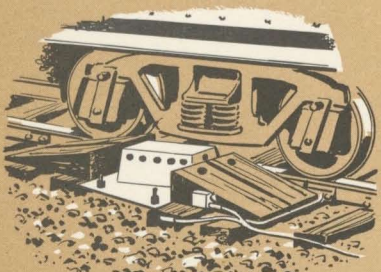
The "hot box" detector's infrared beam, aimed at axles of passing cars, reports instantly any signs of dangerous excess heat.
