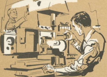
Electronic spectrograph searches lubricating oil samples for microscopic traces of metal that signal excessive engine wear.
