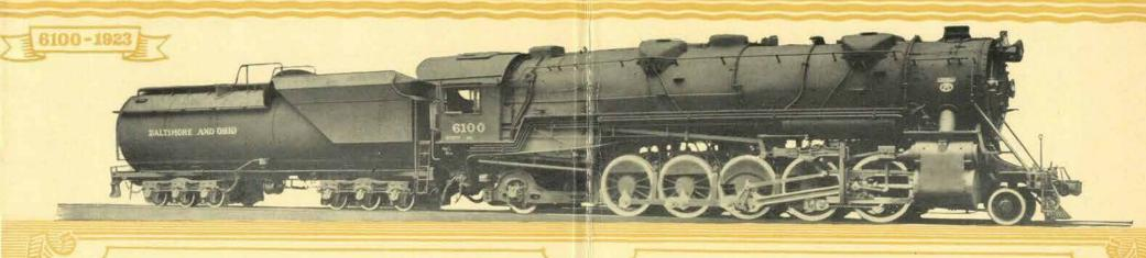
THIS Santa Fe type locomotive was first used on Baltimore and Ohio in 1923. It has power, a reasonable degree of speed and is used in both fast freight and slower movements. With its 64-inch
