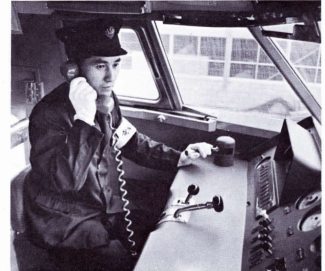
Radio Telephone installed in Motorman's Cab
