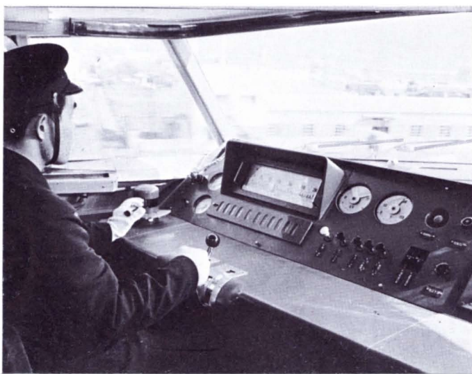
A.T.C. Equipment in Motorman's Cab
