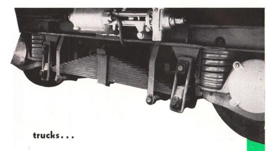
THE DESIGN of the modern trucks of the AGUILA AZTECA is truly an outstanding improvement in railway car construction... These are light in type besides being provided with the double action clasp-brakes with two brake cylinders to each truck, thus making air applications more uniform and potent... Each truck has 8 oil-fed shock absorbers to avoid sudden jolts, and SKF roller bearing system. A very smooth motion is obtained, economizing locomotive exertion...
